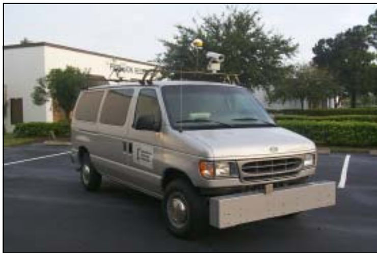
DGPS Receiver supplied with Forward Imaging System for Real-Time Sub-Meter Position Accuracy
