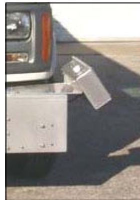
Angled Measuring Laser for 5 Point Rut Depth
